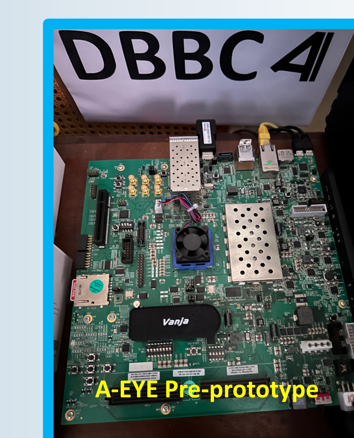
Fig. 7: This controller is a multi-CPU FPGA device optimized will make use of pre-trained neural networks. RFI recognition and mitigation, extraction of non-statistical-noise signals, recognition of human-like extraterrestrial emissions, etc. are the expected applications
