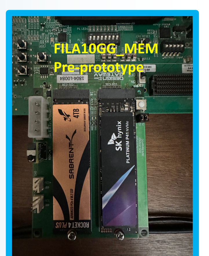
Fig. 8: The FILA100G_MEM is an optional component that provides fast buffered memory for burst-mode operations and direct writing of the received packets on SSD NVMe (PCIe mode) disk modules
