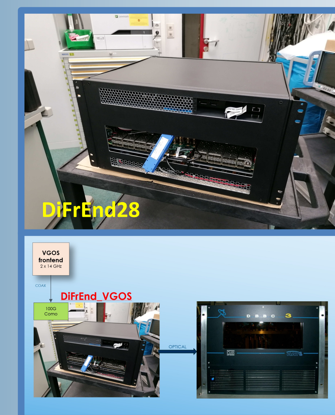
Fig. 4: The ADBCore4 is a key element sampling the signal conditioned by the 100GCoMo and then the digital format of it transferred to the CORE4 FPGA using an aggregate number of serial lines. The required functionality between DSC, OCT, DDC is then processed and kept available to the output channels in order to be sent out to the correlator/recorder or to the FILA100GMEM module
